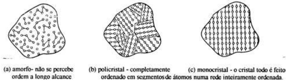
Fig. 10.4- (a) material amorfo; (b) material policristalino; (c) material monocristal.
