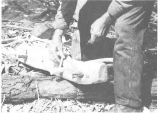
PLATES 74-77 With Mrs. Barnes's and Stan's help, Mr. Barnes selects a small drill and drills two holes—one on the inside end of each bow (*Plate 75*). He then saws off the ends of the bows and, using the scrap, whittles out two hickory pegs (*Plate 76*) and slides them into place (*Plate 77*). These "keys" keep the bows from sliding out.
