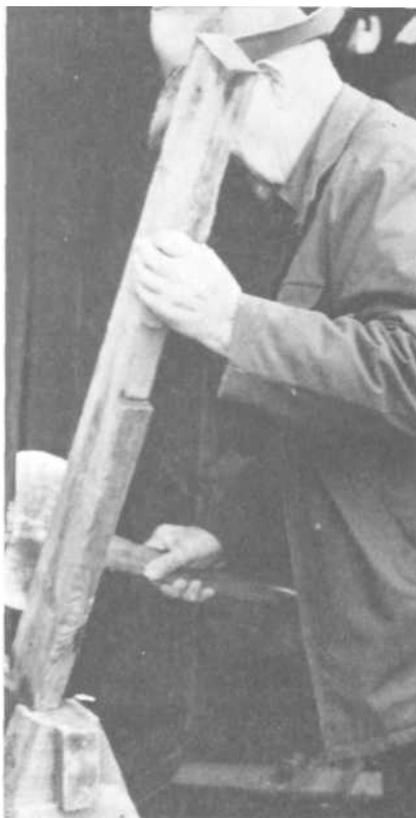
PLATE 171 When the braces for the pedal are in place beside the frame, Greg Strickland drills a hole through both with a brace and bit.
