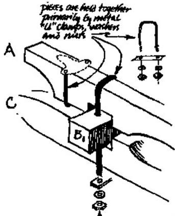
The brake assembly (next page) frames loosely from part B which is bolted firmly to the frounds.
