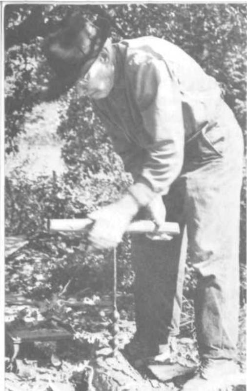
PLATE 65 Roughing out the yoke is a fairly simple process. After the size of the yoke to be made is determined (see diagrams), the sides of a piece of round stock of appropriate size are hewn off leaving a rough-hewn, rectangular block of wood. The outline of the yoke is drawn on the sides using a pattern—if one is available—or measurements. Then, with an auger, the four holes for the bows are drilled from the top surface in the proper places.
