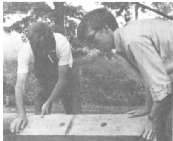
PLATE 129 With the holes drilled, Sam sets the slabs together, drilled sides up, to make sure the holes align properly.
