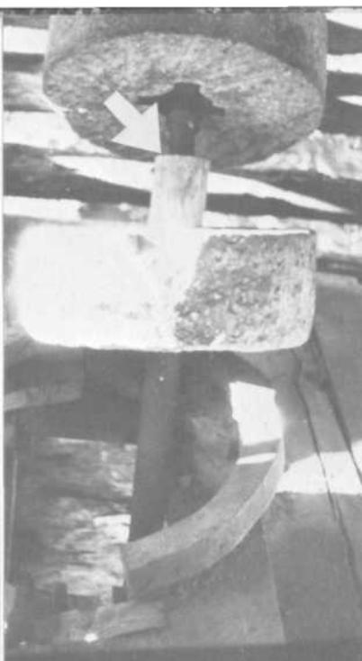
In the photo at left, the bottom millstone has slipped down the shaft exposing the wooden collar (arrow) that prevents meal from falling through the bottom mill's central opening. The bottom stone stays stationary, mounted solidly on the opening on the floor (see also diagram below) while the top stone turns with the shaft. The whole assembly is covered by the circular millstone housing (when operating).
