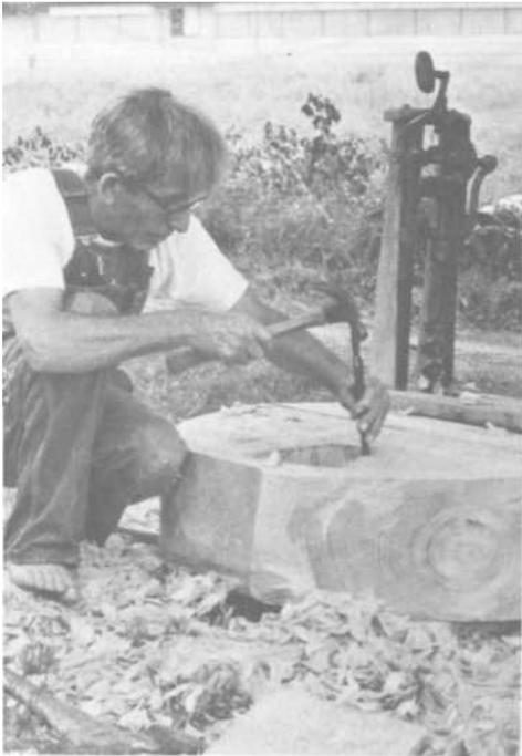
PLATE 141 . . . smooths them up with a hammer and chisel. The holes which he drilled both lighten the work he has to do and act as guides to tell him how deeply into each bucket he may cut without ruining it.
