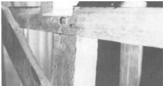
PLATES 261-262 These two photographs show how the frame that holds the heddles (the fifty-two-inch bar) fits down over the top of the loom frame. It is not held in place by anything other than notches.
