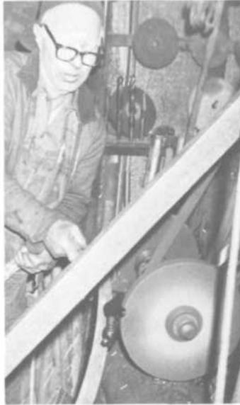
PLATE 110 Now he gets the tire red-hot in his forge. He moves the tire about a foot at a time through the flames until it has gone about four complete, very slow revolutions.
