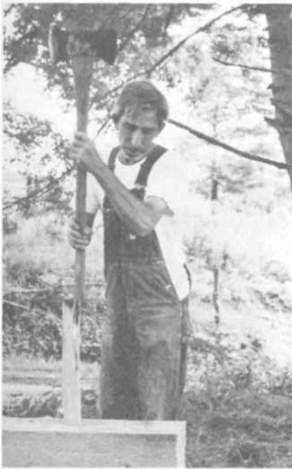
PLATE 131 Next, he drives the pegs into place in one of the two slabs. *Note:* In later steps, when the buckets are being cut out, these pins will be cut into. By that time, however, the two slabs will be held together by two iron hoops.
