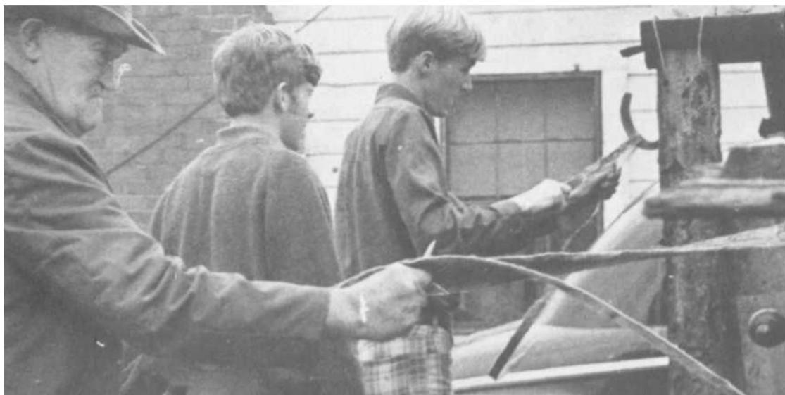
PLATE 170 The frame finished, the foot pedal is now mounted to it. Choose two four-foot 2X4S. Here Minyard sharpens one end of each so they can be driven into the ground. (Note: As in *Plate 171*, they are driven into the ground on a slant, about shoulder width, or  $3/2$  feet, apart.)
