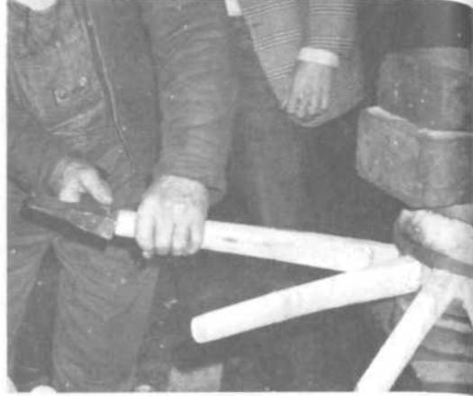
PLATES 96-97 Next the spokes are driven into the mortises in the hub. No nails or glue are needed. The slope of the mortises in the hub automatically creates the required "dish."
