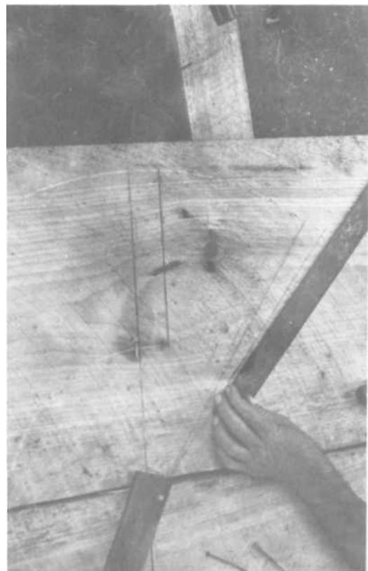
PLATE 136 . . . and the outlines for the first buckets drawn (see measurements in *Plates 152 and 154*).
